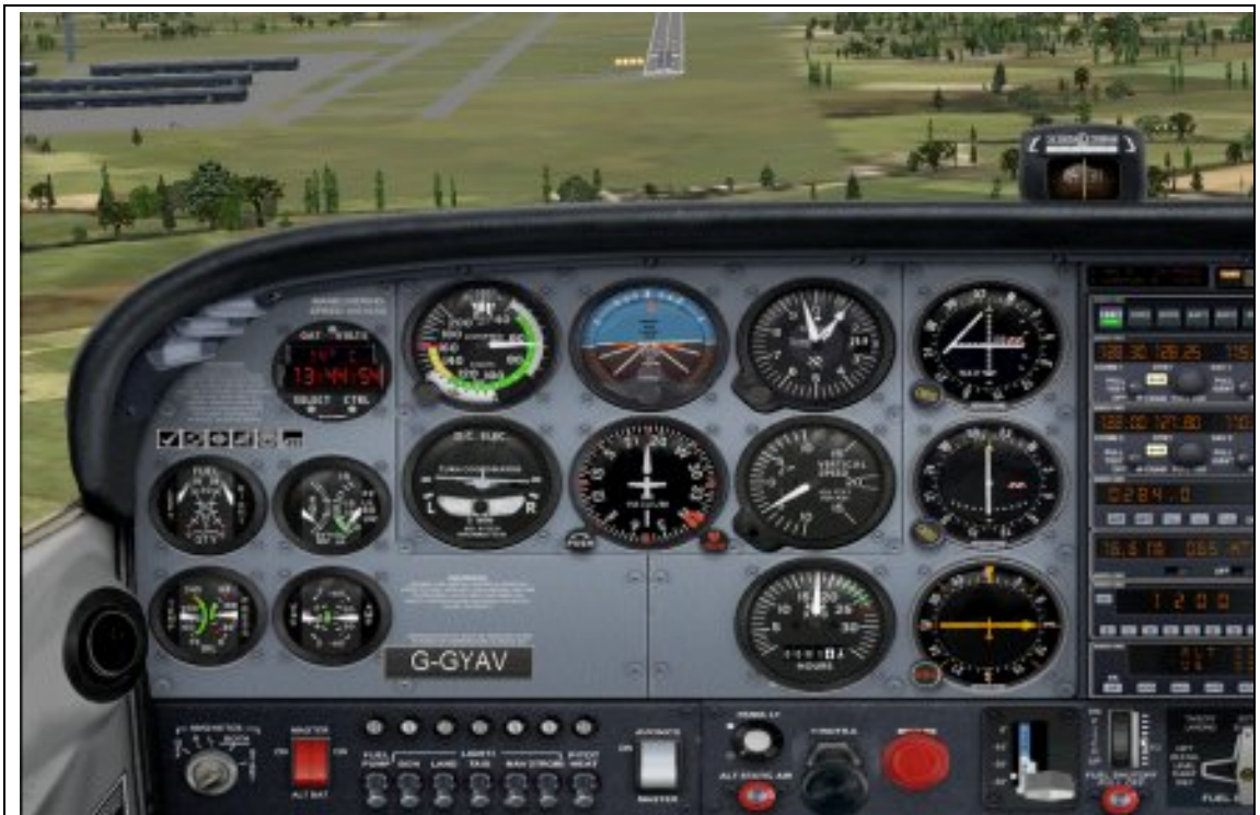
Fig. 5 Powered Descent with Full Flap at Approach Speed
