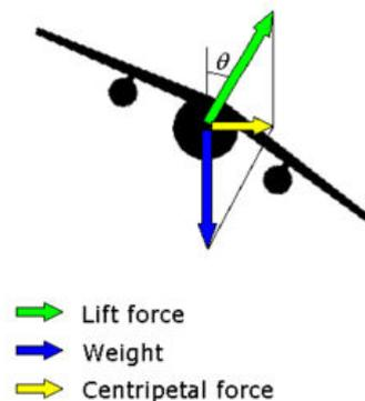
To compensate for this loss of lift, aircraft must either add power to increase airspeed, and therefore lift, or increase lift by increasing the angle of attack of the airflow over the wings by raising the nose. The latter is the technique usually adopted for practical reasons. So in turns, a little back pressure on the yoke or joystick is required.
