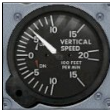
Fig. 1 Vertical Speed Indicator indicating a Climb of 600 Ft per Minute
