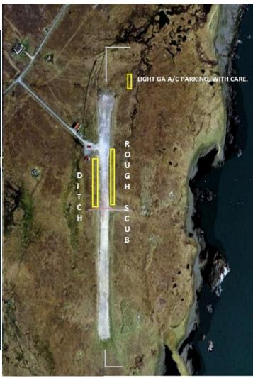
THIS A/F IS NOT RECOMMENDED FOR USE BY A/C WITH SMALL PROPELLER GROUND CLEARANCE, DUE TO THE UNSTABLE HARDCORE SURFACE OF THE RUNWAY AND SURROUNDING GROUND.
