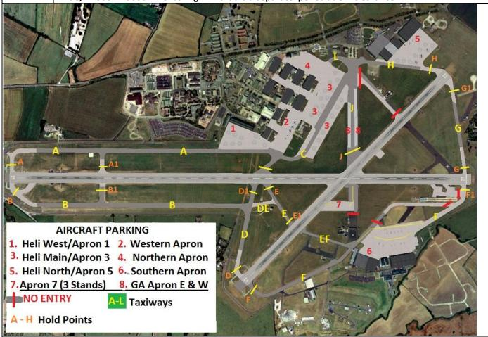
There are no Taxiway Signs on FSX, Only Runway (hold) signs. The hold designators above will be used. NOTE Changes in A/F layout. Taxi M & F (nth of apron 6) CLOSED; access to Apron 7 via Runway intersection. Alert stands, runway 27 threshold. CLOSED. Taxiway EF re-instated, Helicopters and GA ONLY, Taxi J GA ONLY.
